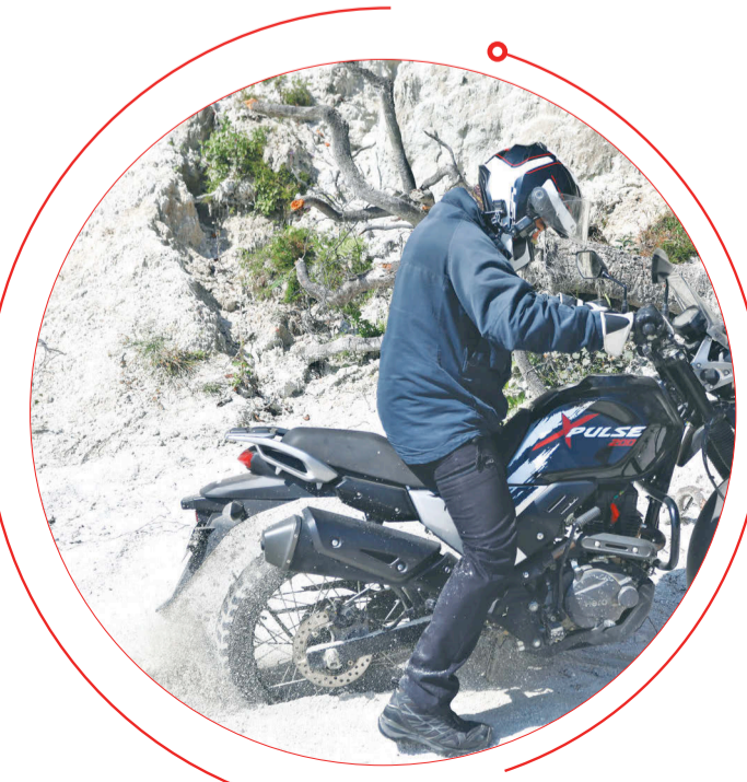
The Xpulse eats potholes for breakfast, thanks to its 190mm front suspension travel. Combined with the 10 step rider-adjustable monoshock, it offers a smooth riding experience.
