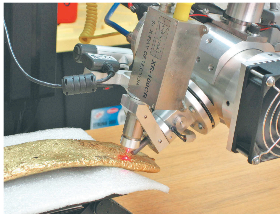
An X-ray detector scans a large gold bar found decades ago in downtown Mexico City.
